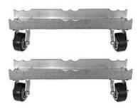
The Mega-Truss Dolly easily holds truss for transport or storage. The 5" aluminum C channel has CNC milled cutouts for truss to ride in. It is important to secure the trusses tightly to the Mega-Truss Dolly with an E-Clip ratchet strap before moving.
